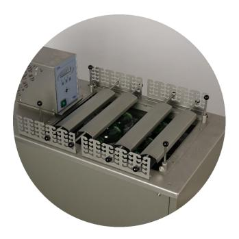
The TLB50 can be used for any test method which require sample preparation prior to the test, like ASTM D323 (Reid Vapor pressure).
